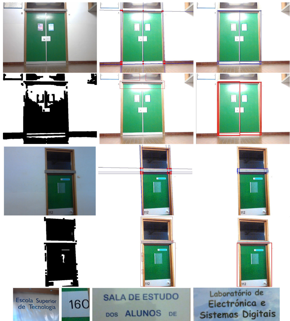
Fig. 5 Frontal doors. Top two rows , from left input image, detected horizontal and vertical edges and intersection points, detected rectangles of method (a), plus segmented image, detected rectangles and selected ones of method (b), and final result. Third and 4th rows another door. Bottom row examples of texts extracted from doors
